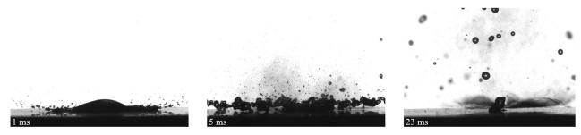
Figure 1: Characteristic behavior of droplet impact on porous heated surfaces in the *partial rebound with breakup* regime.
